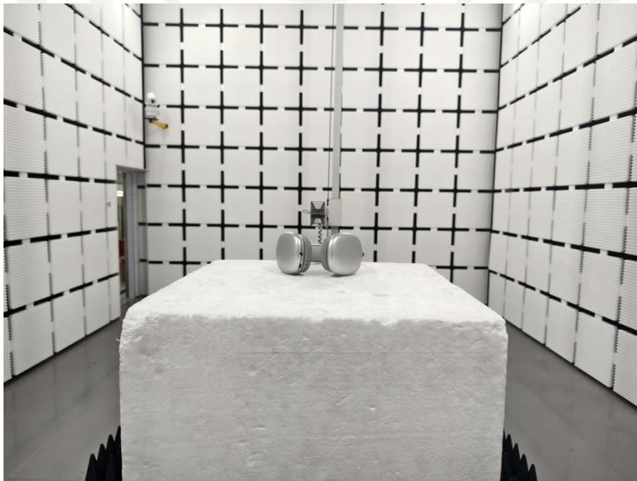
Spurious Radiation Emissions Test (>1G)
