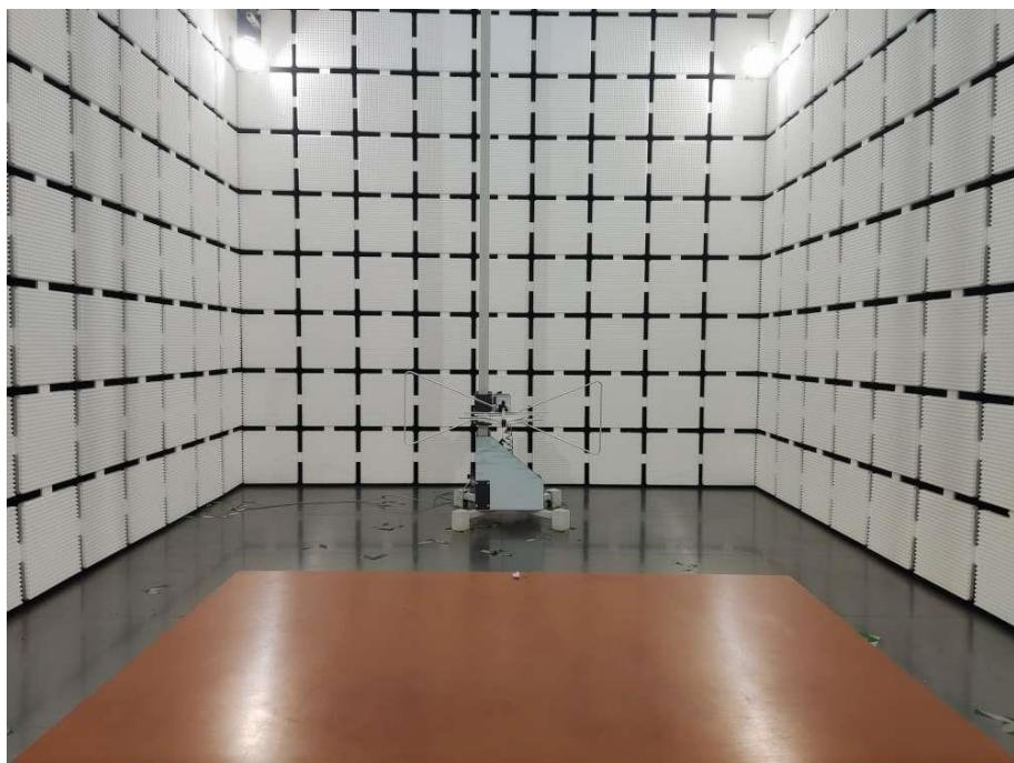
**Radiated Emission Test View 2 (Left earphone)**
