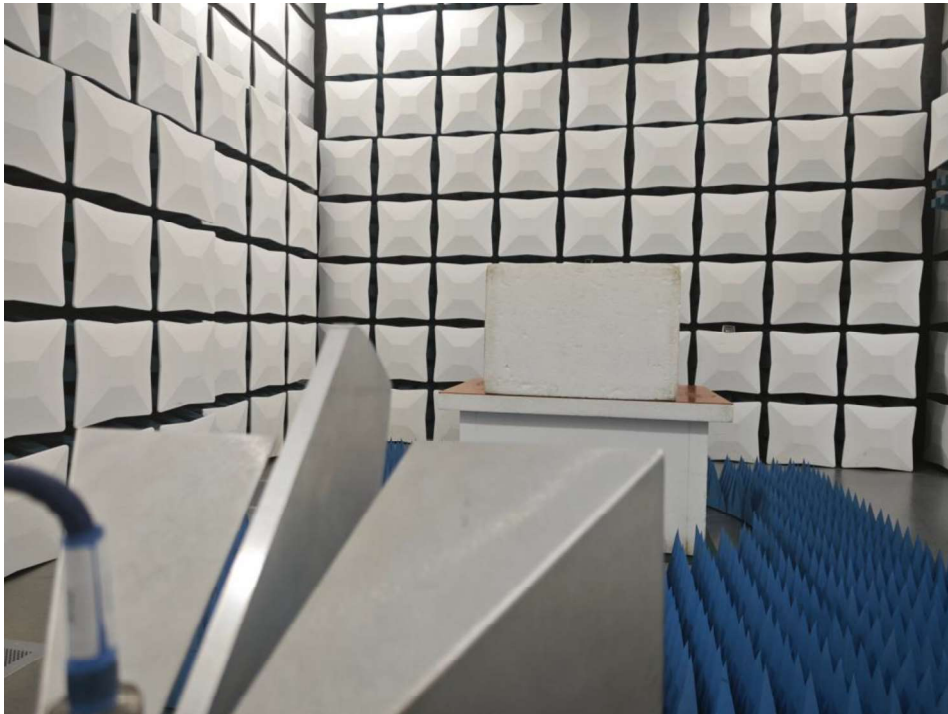
Test Set-up: Radiated spurious emission Above 1GHz
