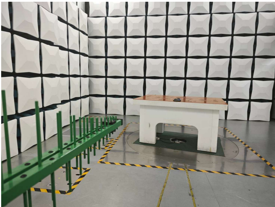
Test Set-up: Radiated spurious emission Below 1GHz
