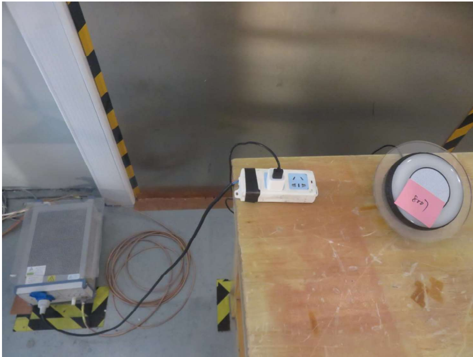
Test Set-up: Conducted emission 150KHz-30MHz
