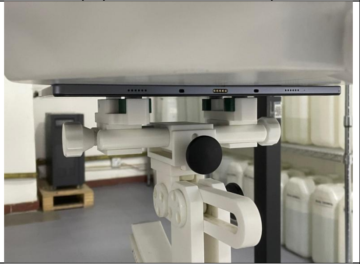
Right Side (Separation distance of 0mm)
