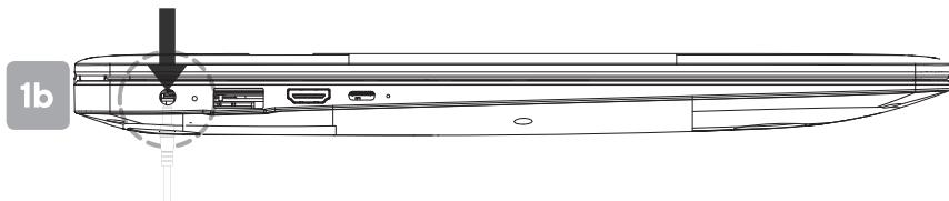
When connected, the laptop will automatically begin to charge. Ensure the battery has been charged for at least 3 hours before using without a power supply for the first time.
