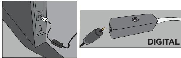
3. Adjust TV audio settings to enable audio out for the port you have plugged the transmitter into. You may have the option to mute the sound coming from the internal TV speakers or keep both on. We recommend keeping both on if you have the option so you don't have to switch back and forth. For **SendXDigital**, you will need to select the PCM 2-channel option only if it is shown as an option.
