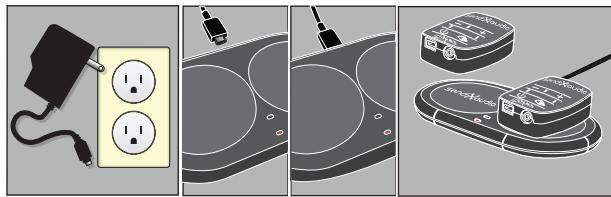
2. Connect transmitter to TV and plug **USB** into power source on TV
