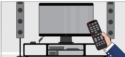
5. Turn on the **SendXfobs** once they are charged. Ensure that the LED light for the "Mode" on the **SendXFob** is set to receive mode ("Recv"). You can depress the **Mode** button to set the **SendXFob** to receive mode if it is in **Send** mode. Press the **Bond** button twice to search for the audio signal being transmitted from the TV.
