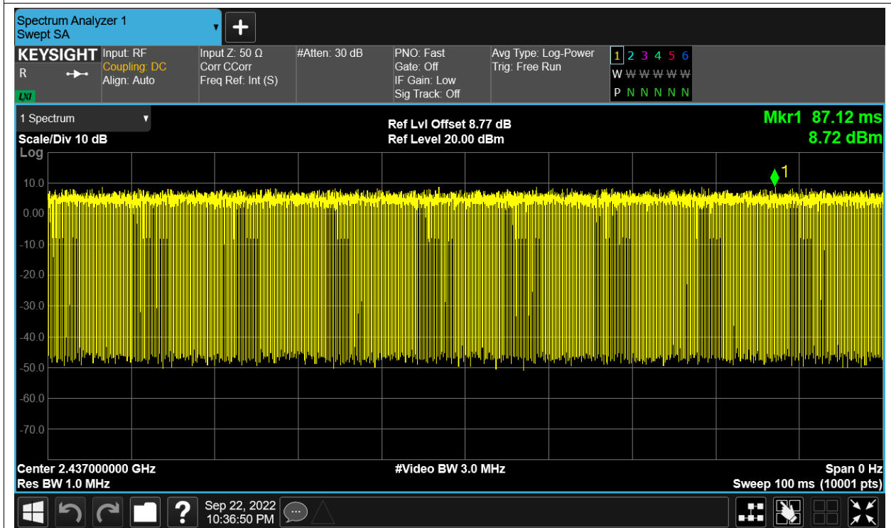
Duty Cycle NVNT n20 2462MHz Sum
