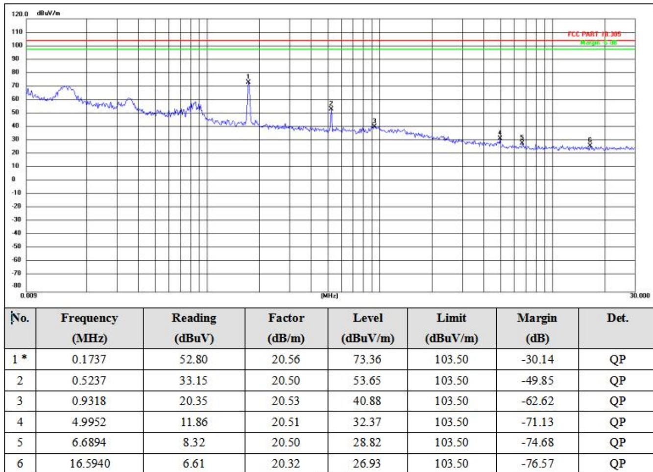
Remark: Measured at antenna position 0 degree and 90 degree, recorded worst case at 0 degree.
