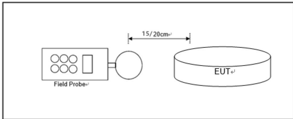
Note: Measurements should be made from all sides and the top of the primary/client pair, with the 15/20 cm (the top is 20cm, and the other five sides are 15cm) measured from the center of the probe(s) to the edge of the device.
