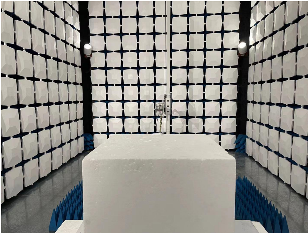
Above 1GHz for radiated emission test setup
