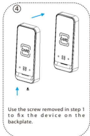
Use the screw removed in step 1 to fix the device on the backplate.
