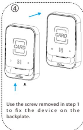
Use the screw removed in step 1 to fix the device on the backplate.
