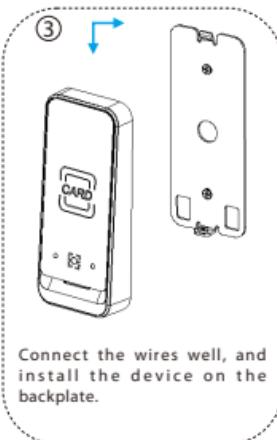
Connect the wires well, and install the device on the backplate.
