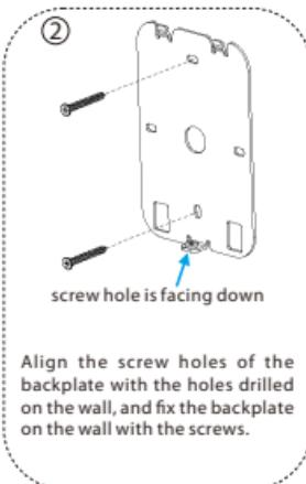
Align the screw holes of the backplate with the holes drilled on the wall, and fix the backplate on the wall with the screws.
