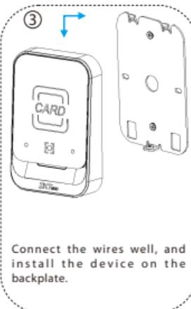
Connect the wires well, and install the device on the backplate.
