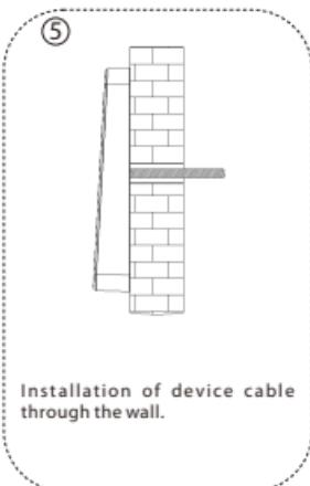
Installation of device cable through the wall.
