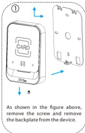
As shown in the figure above, remove the screw and remove the backplate from the device.
