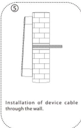
Installation of device cable through the wall.
