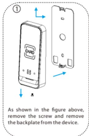
As shown in the figure above, remove the screw and remove the backplate from the device.
