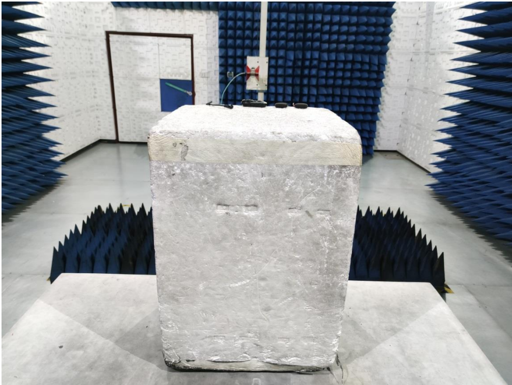
RADIATED EMISSION TEST SETUP ABOVE 1GHZ
