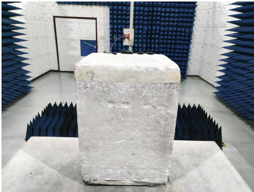
RADIATED EMISSION TEST SETUP ABOVE 1GHZ
