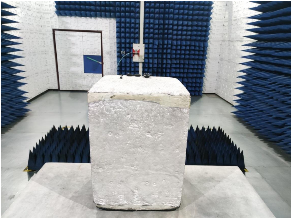
RADIATED EMISSION TEST SETUP ABOVE 1GHz
