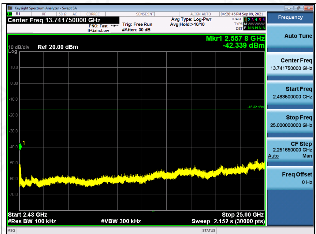
Test_Graph_EDR_ANT1_2402_3Mbps_Higher Band Emissions
