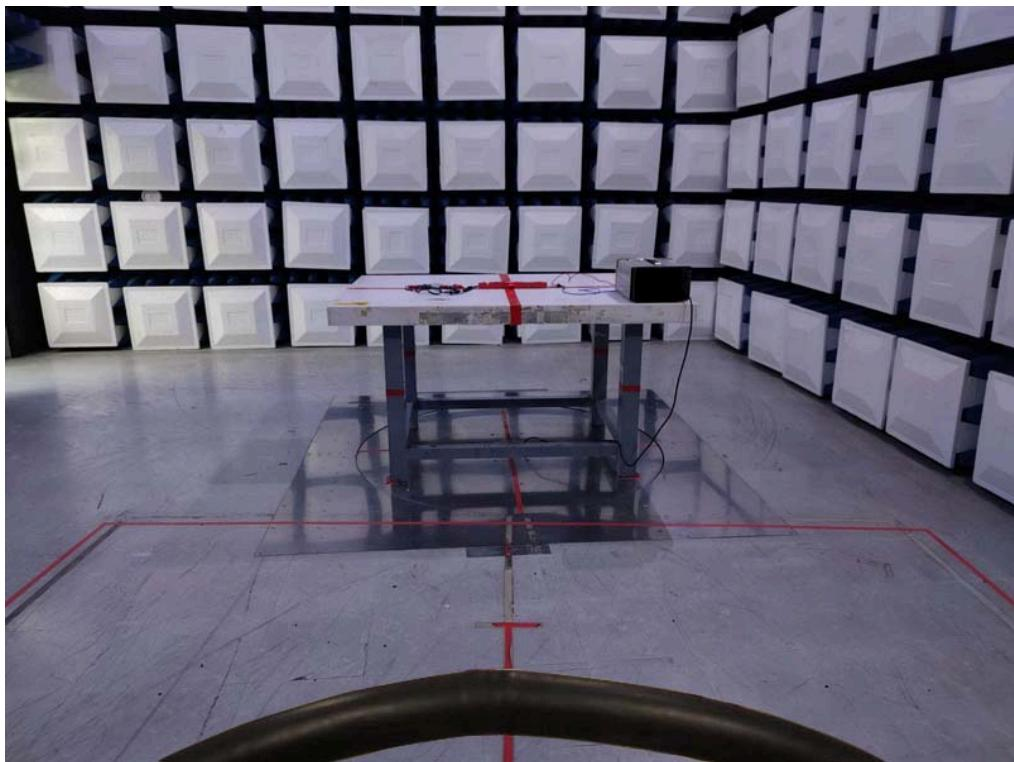
**Radiated Emissions Test Photos****30 MHz to 1 GHz**
