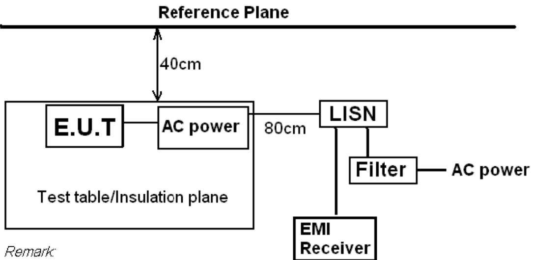
*Remark:**E.U.T: Equipment Under Test**LISN: Line Impedance Stabilization Network**Test table height=0.8m*
