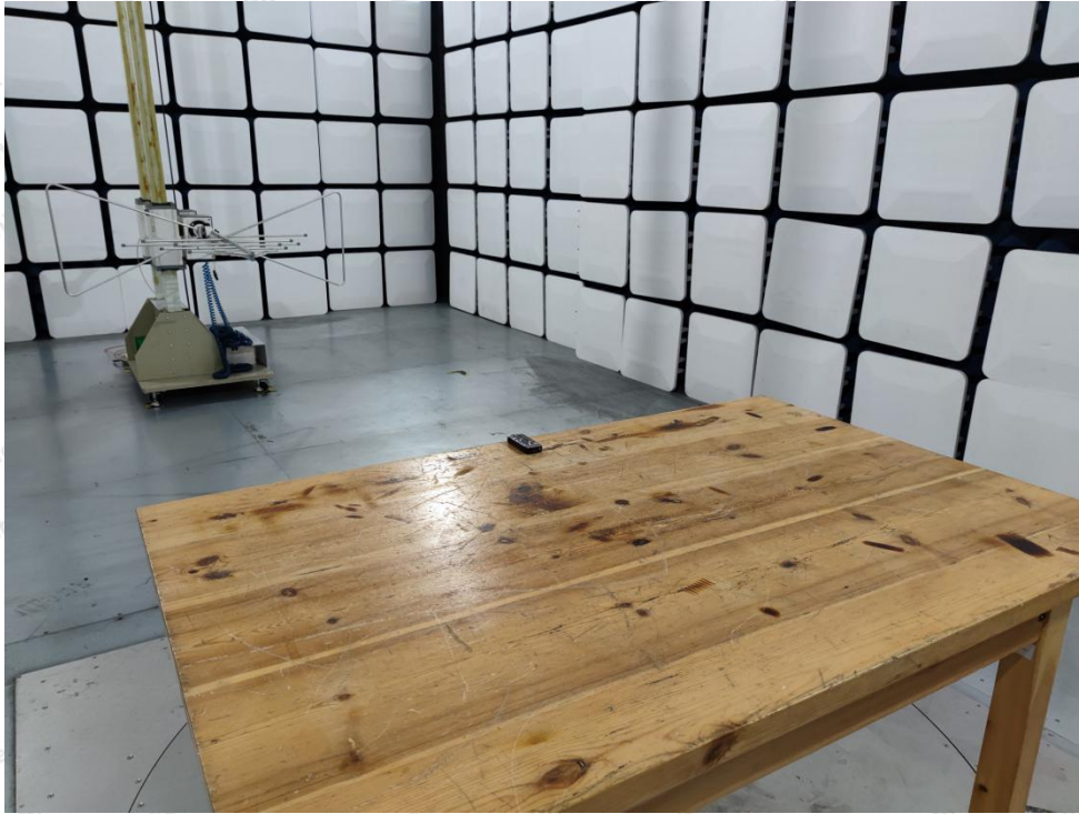
Photo of Radiation Emission Test
