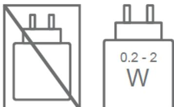
The power delivered by the charger must be between min 0.2 Watts required by the radio equipment, and max 2 Watts in order to achieve the maximum charging speed.
