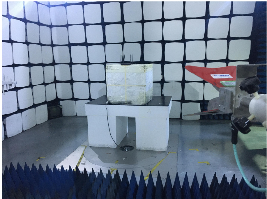
Radiation Emission Test Setup (1GHz to 18GHz)
