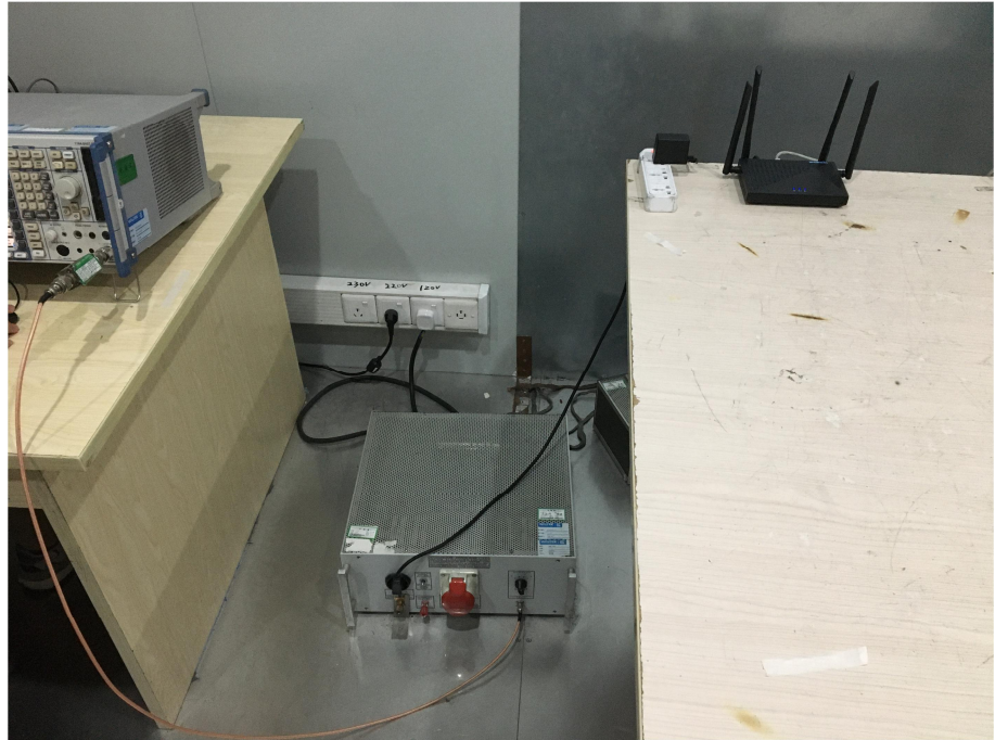
Conducted Emission Test Setup
