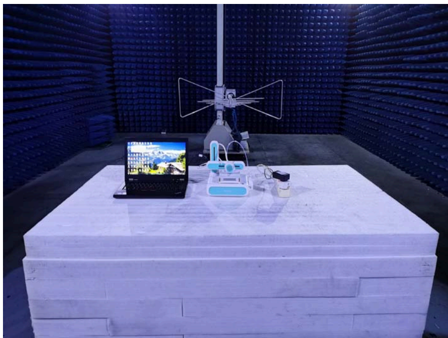
Photo of Radiated Emission Measurement (Below 1G)
