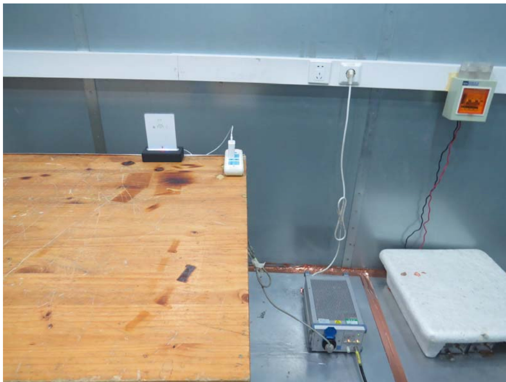
Picture 2 Conducted Emission Test Setup
