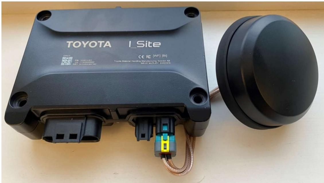
Picture showing the Toyota DHU4 unit to the left. Connected with a four-port mini-fakra to the Smarteq antenna to the right.
