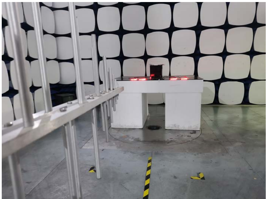
Radiation Emission Test Setup (30MHz to 1GHz)
