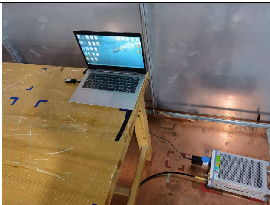
Conducted Emissions Test Setup (with charger)
