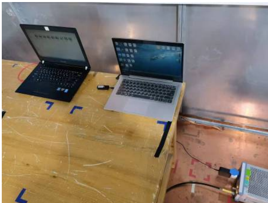
Conducted Emissions Test Setup
