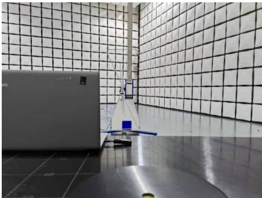
Radiated Emissions Test Setup (30-1000MHz)
