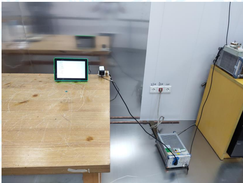
Photo of Setup for Conducted Emission
