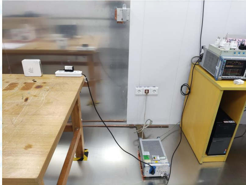
Photo of Setup for Conducted Emission
