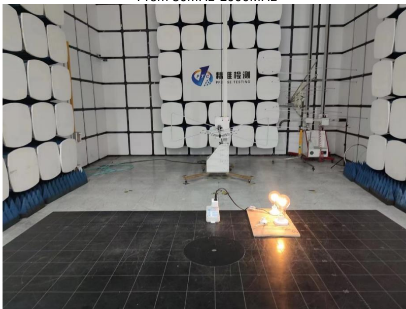
Radiated Spurious Emissions From 30MHz-1000MHz
