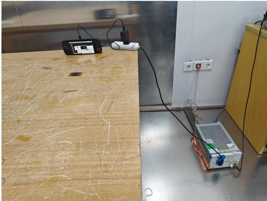
Photo of Setup for Conducted Emission
