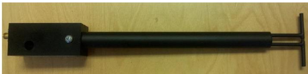
Figure 1 – MVG COMOSAR Validation Dipole
