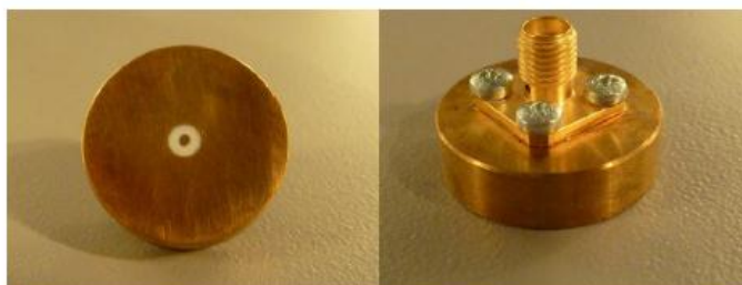
Figure 1 – MVG LIMESAR Dielectric Probe
