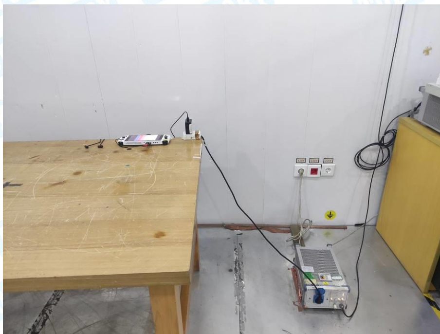
Photo of Setup for Conducted Emission
