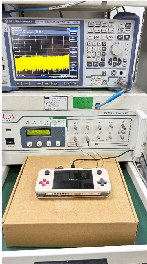
Photo of Setup for RF Conducted
