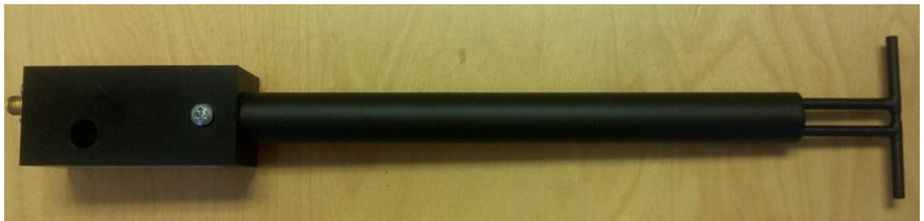
Figure 1 – MVG COMOSAR Validation Dipole
