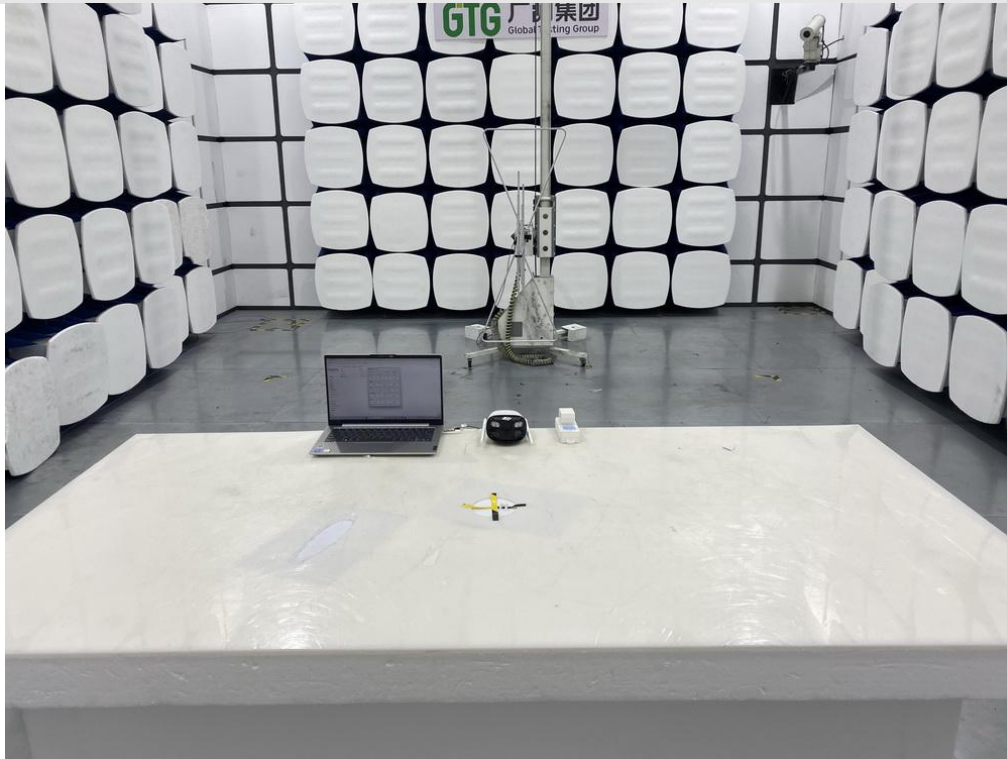
Radiated emissions below 1GHz
