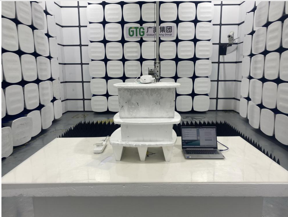
Radiated emissions above 1GHz
