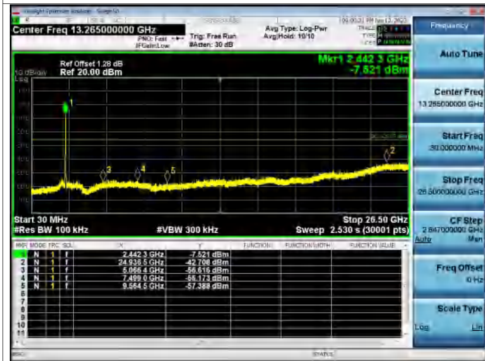
Tx. Spurious NVNT n40 2437MHz Ant1 Emission
