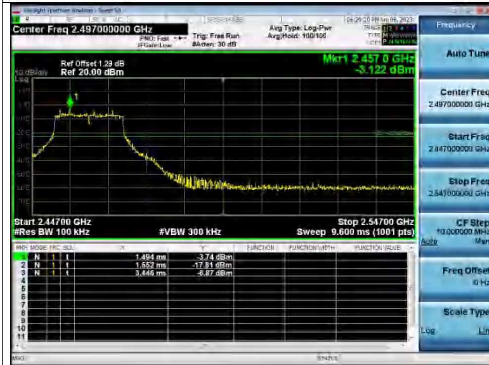
Band Edge NVNT g 2462MHz Ant1 Emission
