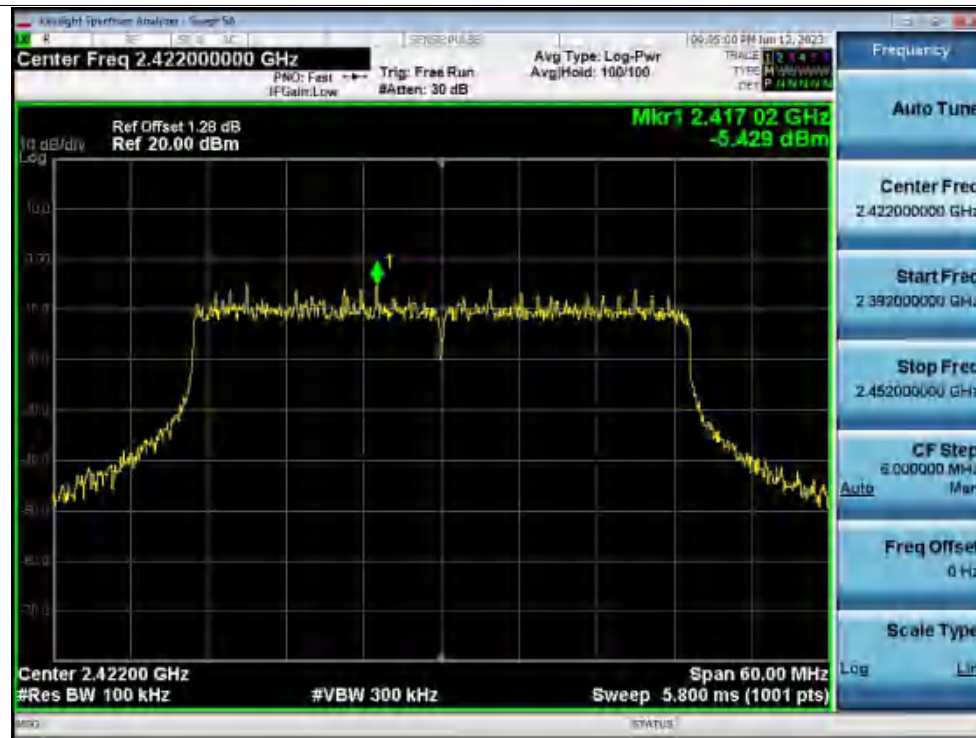
Tx. Spurious NVNT ax40 2422MHz Ant1 Emission
