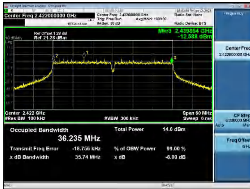
-6dB Bandwidth NVNT n40 2422MHz Ant1
