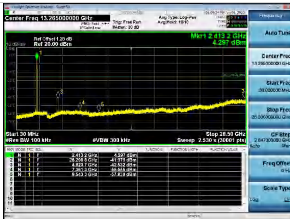
Tx. Spurious NVNT b 2412MHz Ant1 Emission
