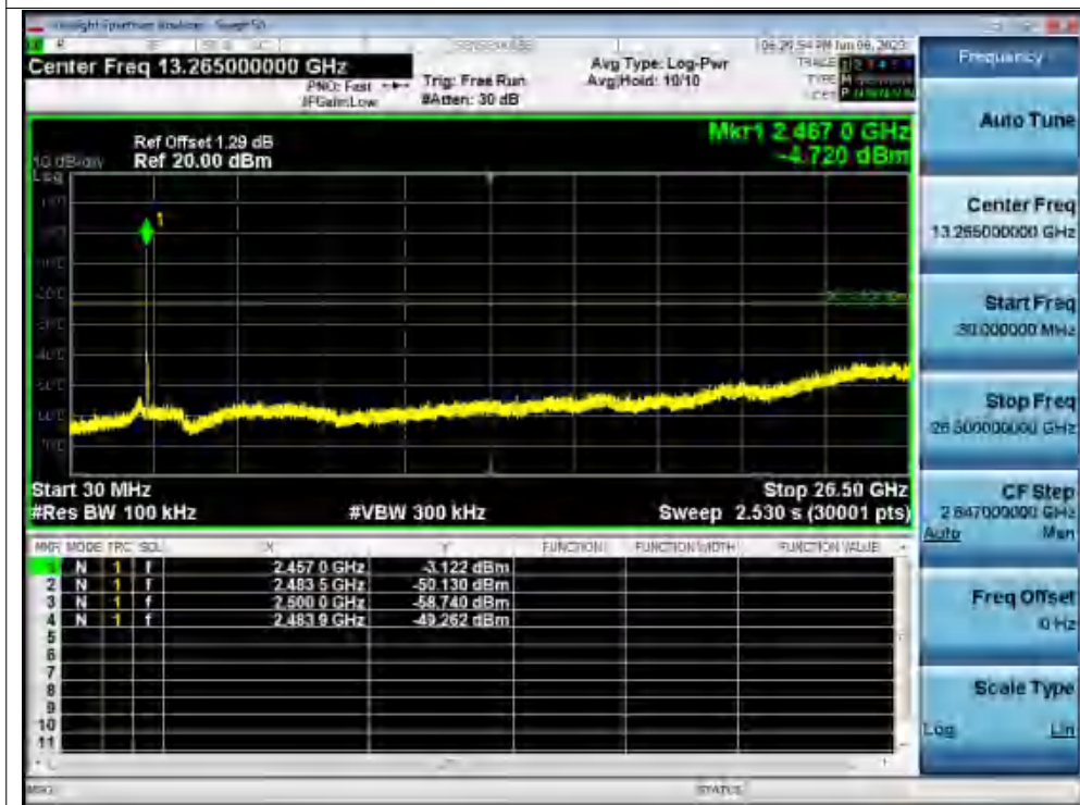
Tx. Spurious NVNT g 2462MHz Ant1 Emission
