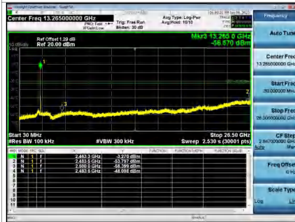
Tx. Spurious NVNT n20 2462MHz Ant1 Emission
