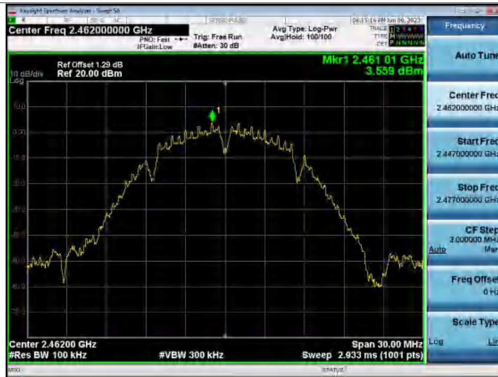
Tx. Spurious NVNT b 2462MHz Ant1 Emission
