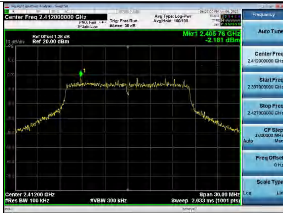
Tx. Spurious NVNT g 2412MHz Ant1 Emission
