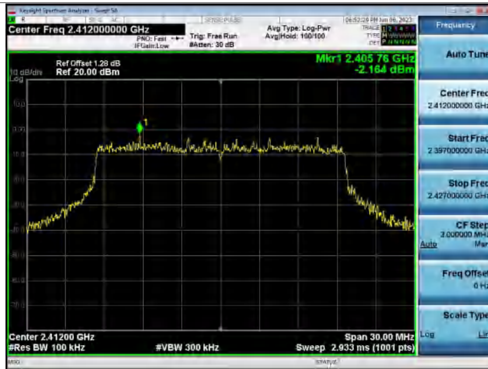
Tx. Spurious NVNT ax20 2412MHz Ant1 Emission
