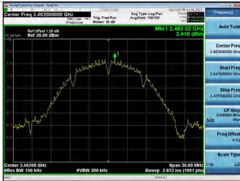
Band Edge NVNT b 2462MHz Ant1 Emission
