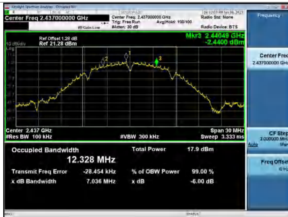
-6dB Bandwidth NVNT b 2437MHz Ant1
