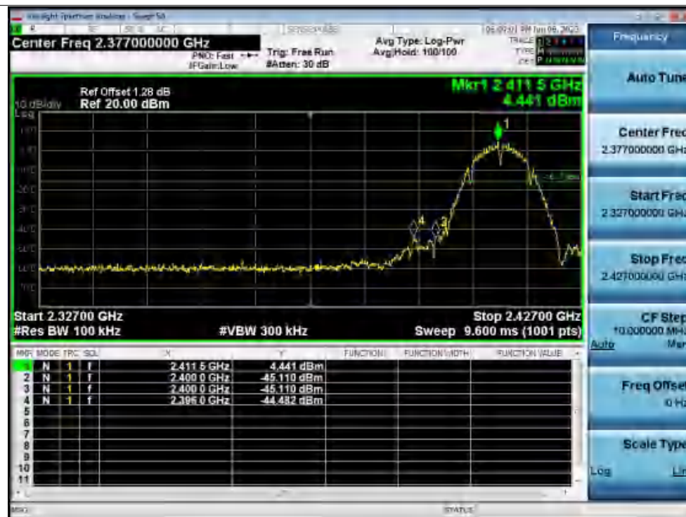
Band Edge NVNT b 2412MHz Ant1 Emission
