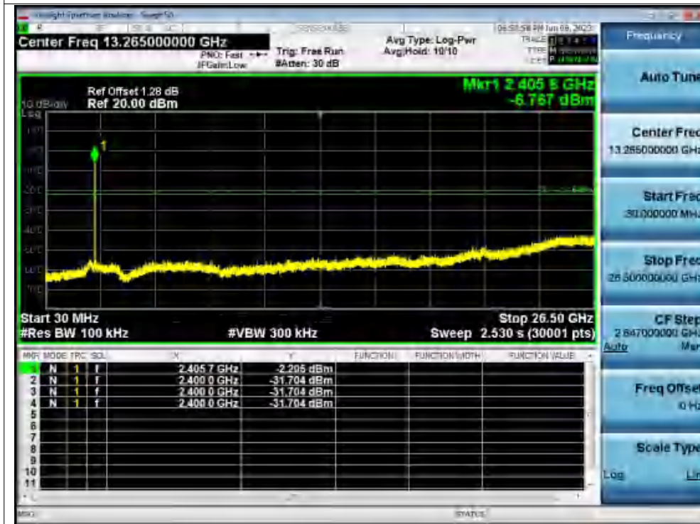
Tx. Spurious NVNT ax20 2412MHz Ant1 Emission
