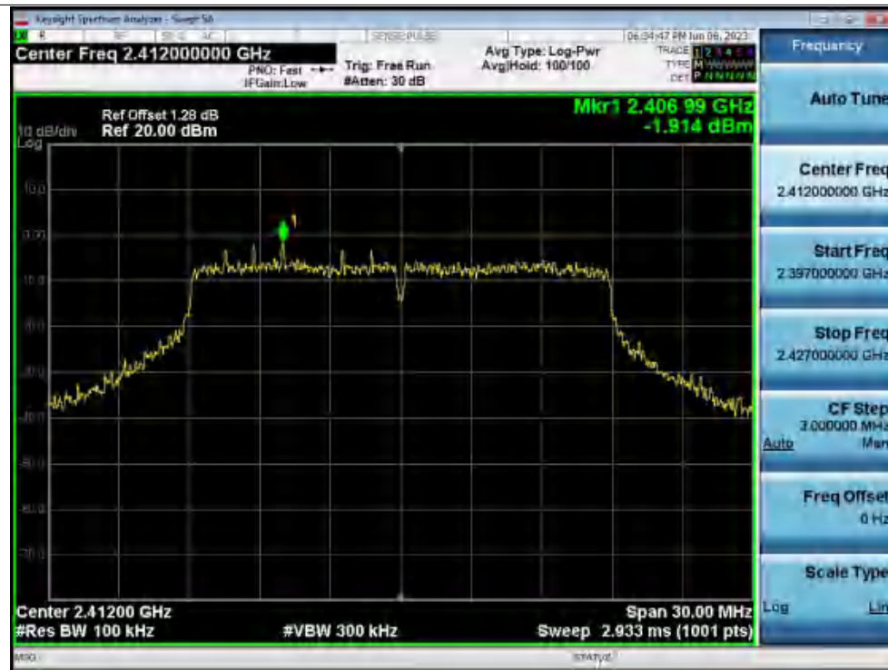
Band Edge NVNT n20 2412MHz Ant1 Emission
