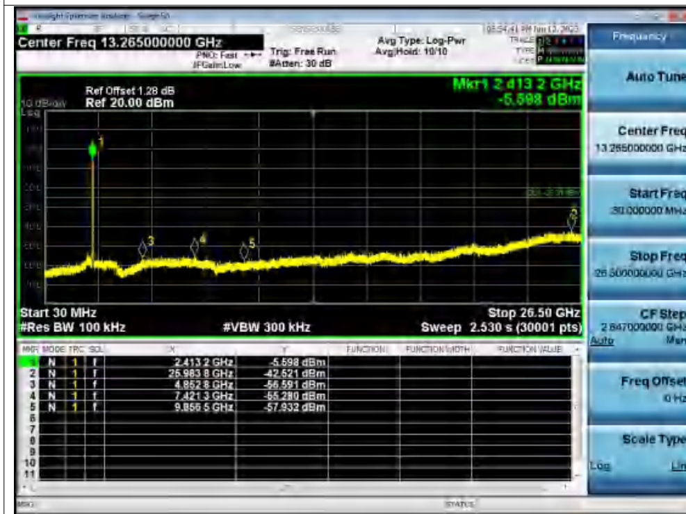
Tx. Spurious NVNT n40 2422MHz Ant1 Emission
