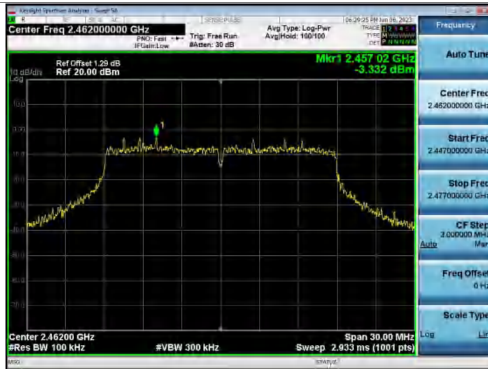
Tx. Spurious NVNT g 2462MHz Ant1 Emission
