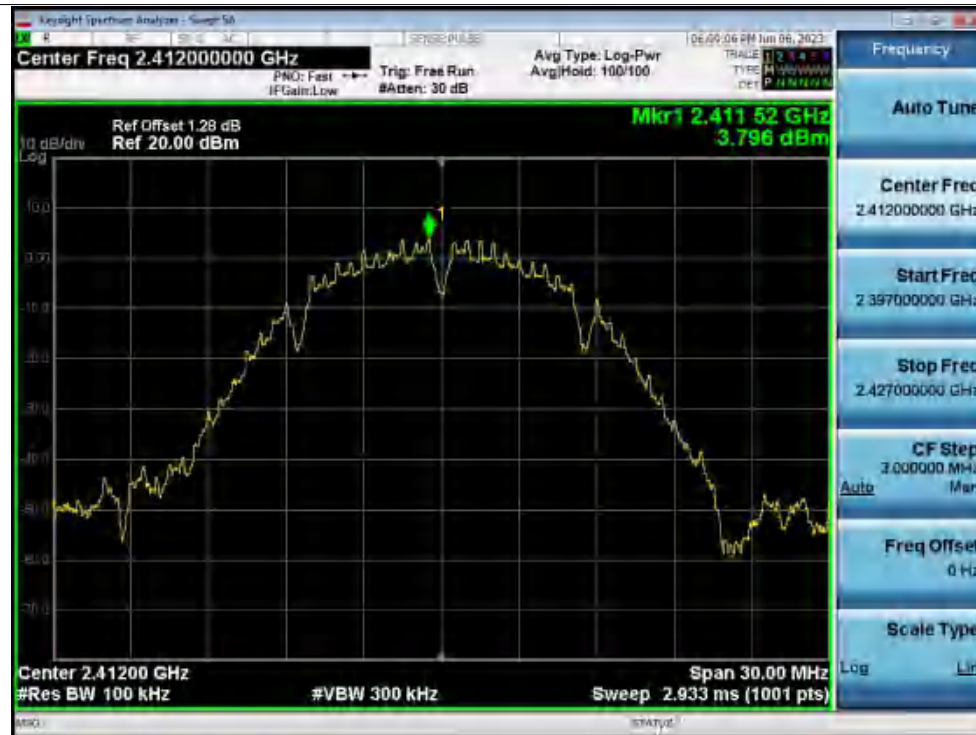
Tx. Spurious NVNT b 2412MHz Ant1 Emission
