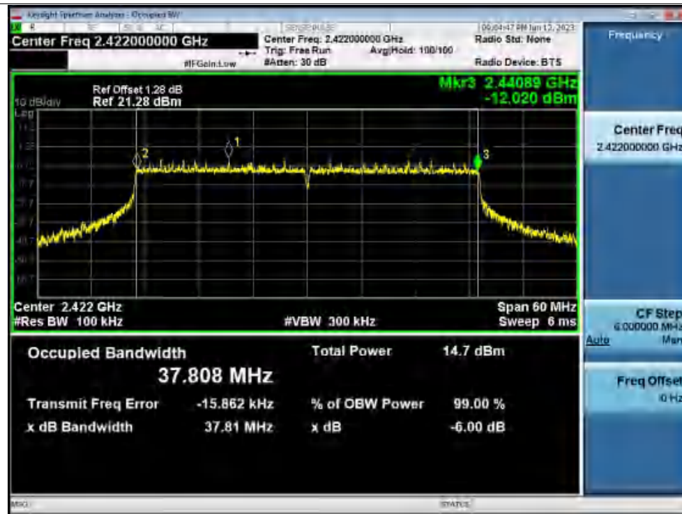
-6dB Bandwidth NVNT ax40 2422MHz Ant1
