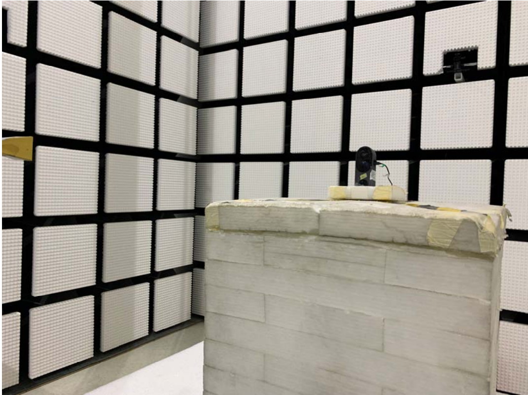
Radiated Emission Above 90-100GHz View
