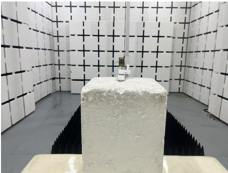
Set-up for Radiated Spurious Emission, Above 1GHz
