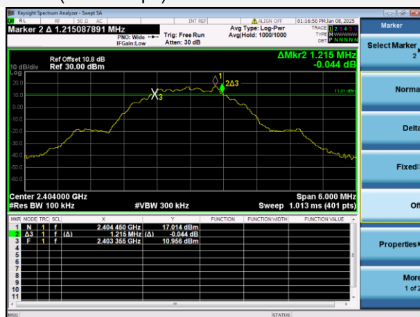
GFSK (BLE 2Mbps) LOW CHANNEL
