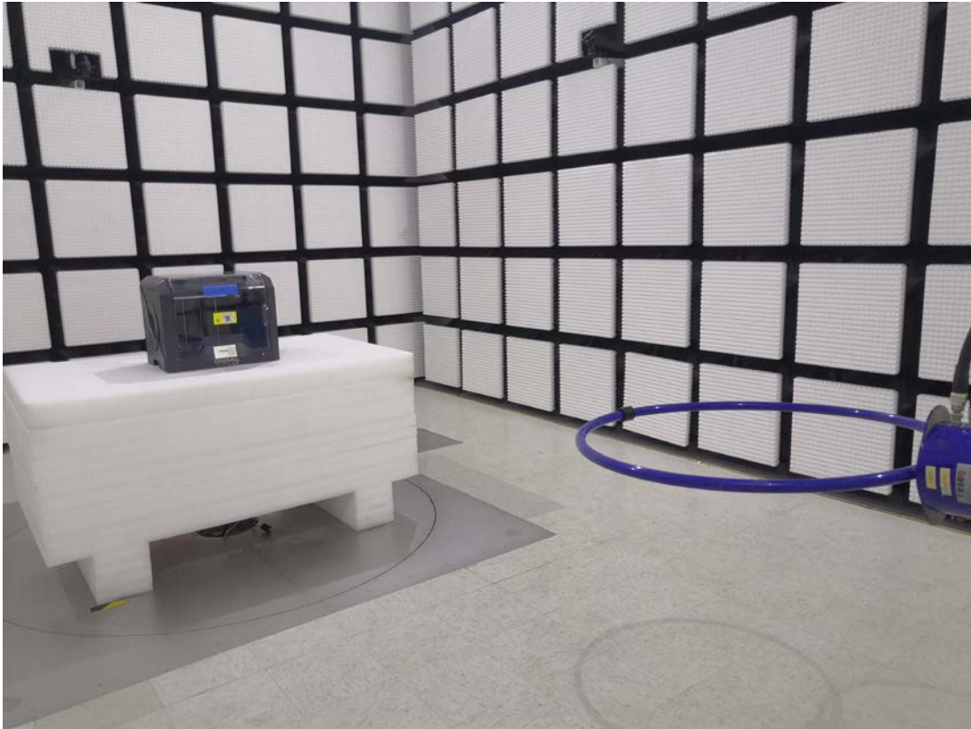
Radiated Emission 30MHz~1GHz View
