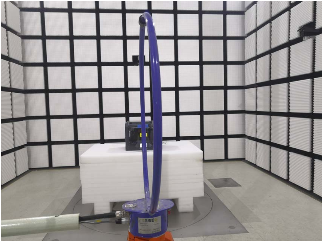
Radiated Emission 9kHz~30MHz View Perpendicular
