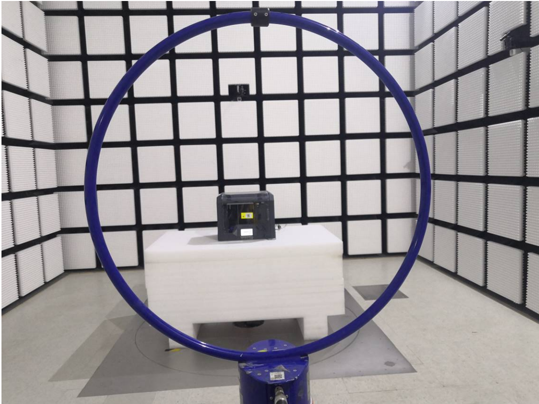
Radiated Emission 9kHz~30MHz View Perpendicular
