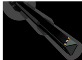
Figure 5-3 Triangular Probe Configuration
