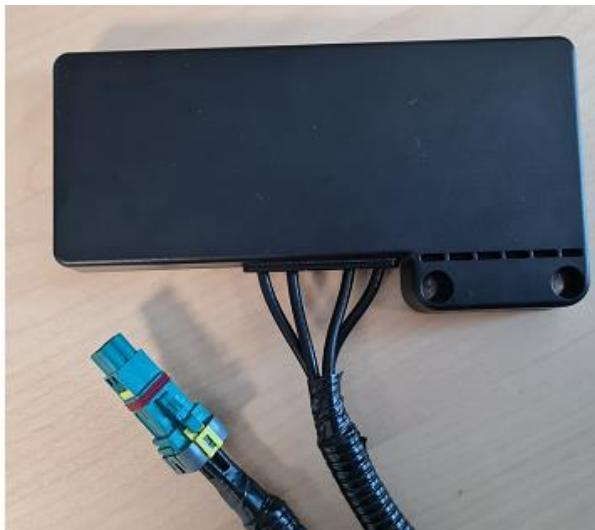
Picture showing the Toyota DHUnx unit to the left. Connected with a four-port mini-fakra to the Molex antenna to the right.
