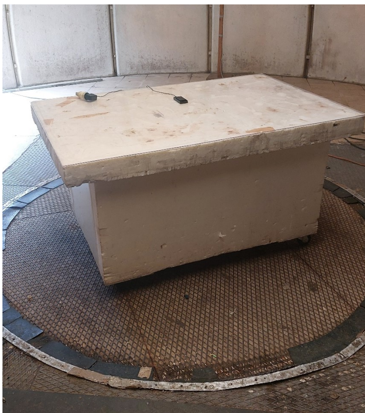
Measurement of radiated disturbances.
