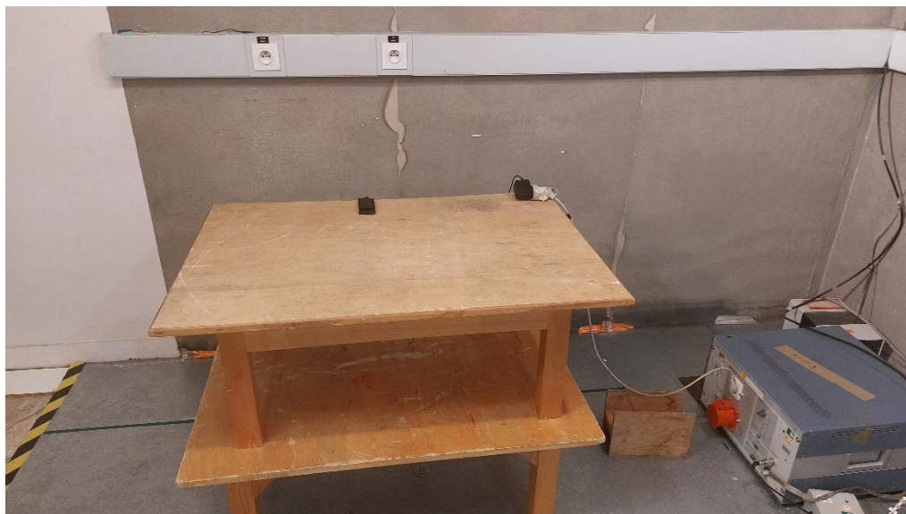
Test set up of conducted emission on power supply
